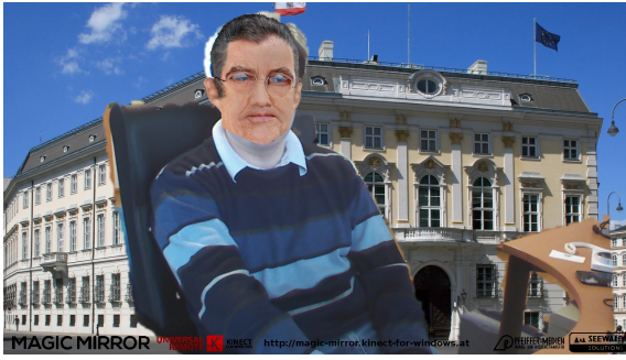
Figure 5: Kinect V1 – Sample Image. We used a z-filter with adjustable distance here where all objects beyond a certain distance were replaced by background. This accounts for the presence of the chair and parts of the table in this image. Later we implemented z-Skeleton filtering which replaced all background except for recognized bodies (skeletons in Kinect terminology).
